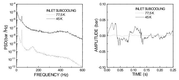
Figure 3. - Pressure Sensor P2X Signal in Frequency and Time Domain - ONB Condition.
