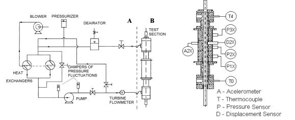
Figure 2. - Experimental Loop for Subcooled Boiling - Flow Diagram and Test Section.
