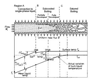
Figure 1 - Schematic Representation of the Subcooled Boiling Regimen.
